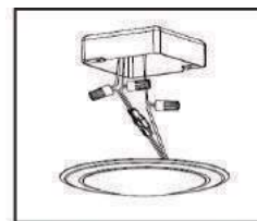
1. Wire the connector to house wiring and attach to fixture
